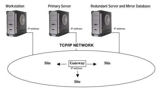
The Redundant Server monitors the communication between itself and the Primary Server. The Mirror Database is a real-time copy of the system database and Windows system registry entries.
