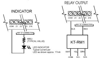
**Note**: May require a KT-PC4204 power supply module if drawing too much current from the Combus.
