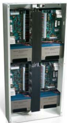
28-inch Multi-Door Controller Kit shipped with 2 KT-300 controllers. Image shown fully configured.
