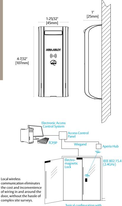
Typical configuration with electromagnetic lock
